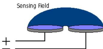
If the dielectric remains constant, the capacitance also remains constant. If the dielectric changes, the capacitance naturally also changes.
